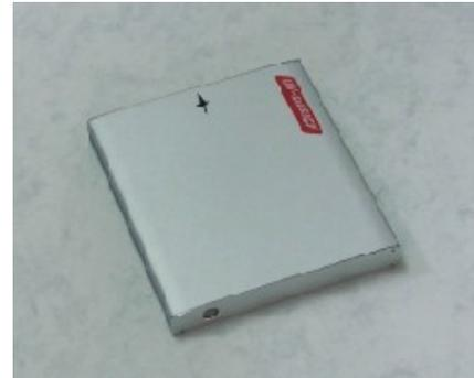
The VOC Data Sampler 822 is a portable, pass-through, Pocket-PC based data logger for IR, convection and other heat curing systems using solvent containing inks, glues, lacquers and paints. It is detecting organic solvent vapours, other volatile vapours and combustible gases such as carbon monoxide, ethanol, isobutanes, n-hexanes, benzenes, ethanol, acetone etc.
